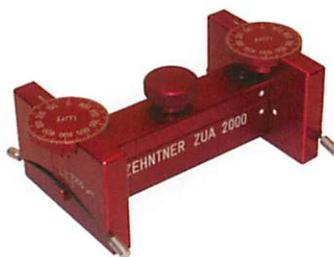
The first cross-cut tester with flexible cutting head for cutting head for even, reproducible cross-cuts.
