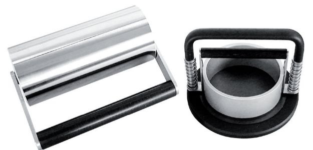
COBB-TESTER with separated couch roll
