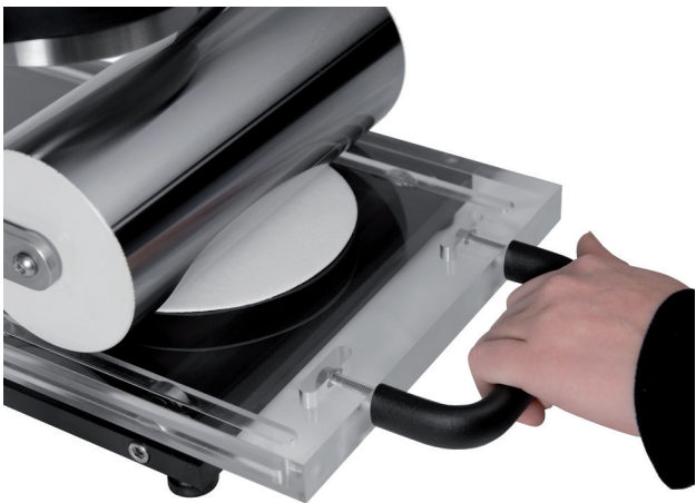
Couching by moving the couching plate
