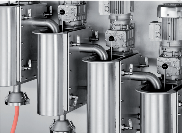
Classifier container with quick clamping device
