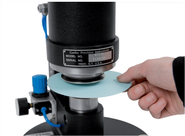
Sample is pneumatically clamped when the start button is pressed
