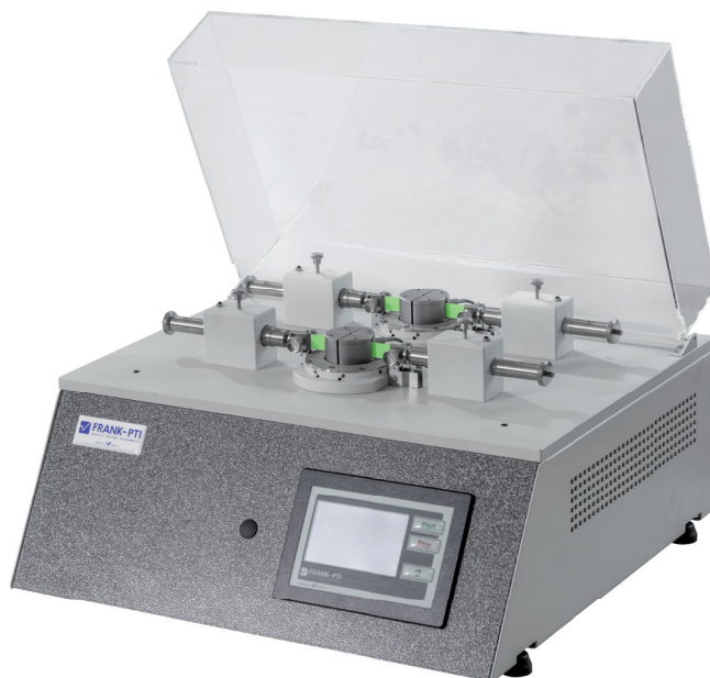
Folding unit with open security cover
