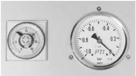
Timer watch and vacuum control for the dryers
