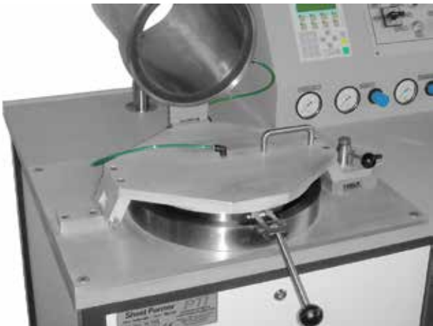
Pneumatic couching device
