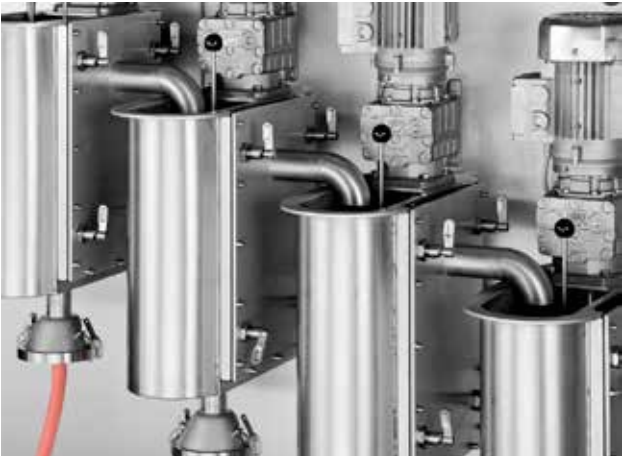
Classifier container with quick clamping device
