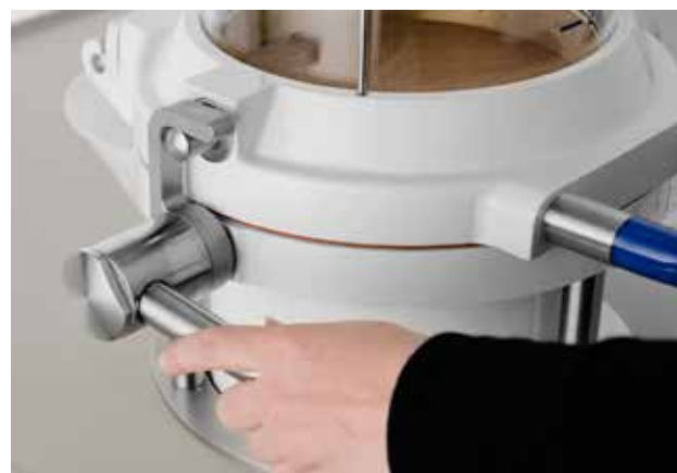
Opening the former column by lifting the handle
