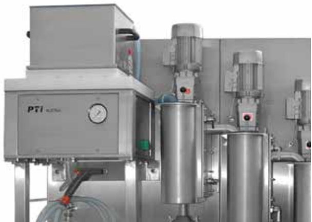
Bauer McNett Fibre classifier with built-on Somerville
