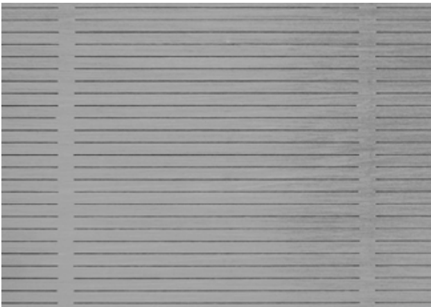
Standardised slot plate with a slot size of 0,15 x 45 mm
