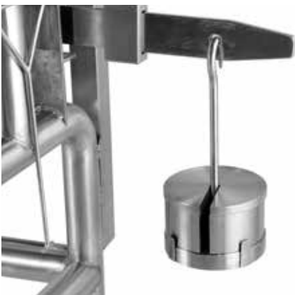
Beating pressure adjustable by means of a weight
