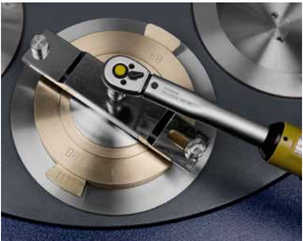
Closing the grinding vessel sets with a torque wrench
