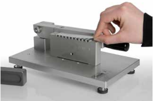
An adhesive tape is applied to the flute
