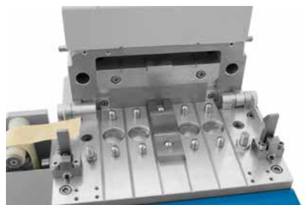
Open sample preparation station for placing the test samples
