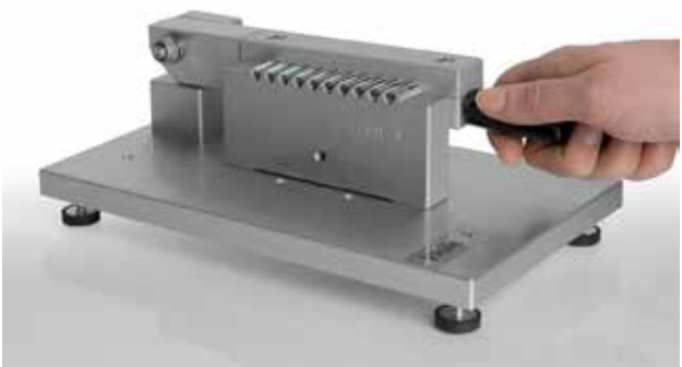
The flute is placed into the "Third hand" and clamped
