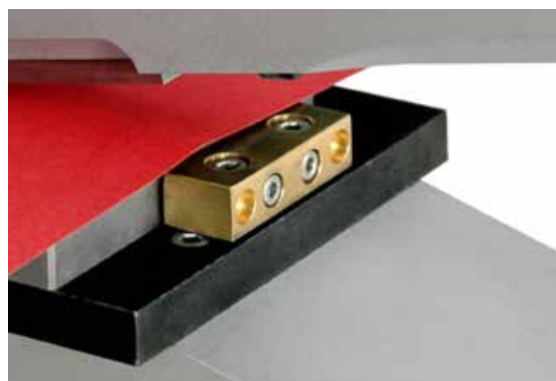
The material to be punched is placed on the lower blade
