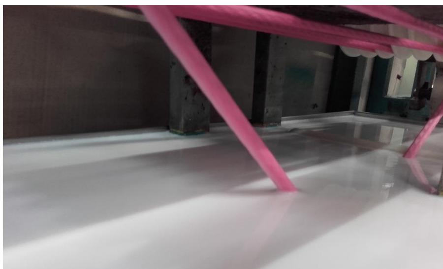
soaking of rope into the coating mixture
