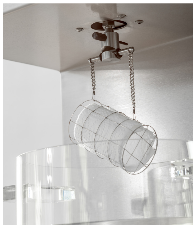
Immerse basket and exchangeable water container
