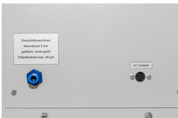
Rear panel of device with supply connections
